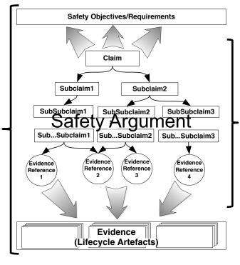
• Safety argument is the "spine" of the safety case showing how safety objectives/ requirements are connected with evidence
