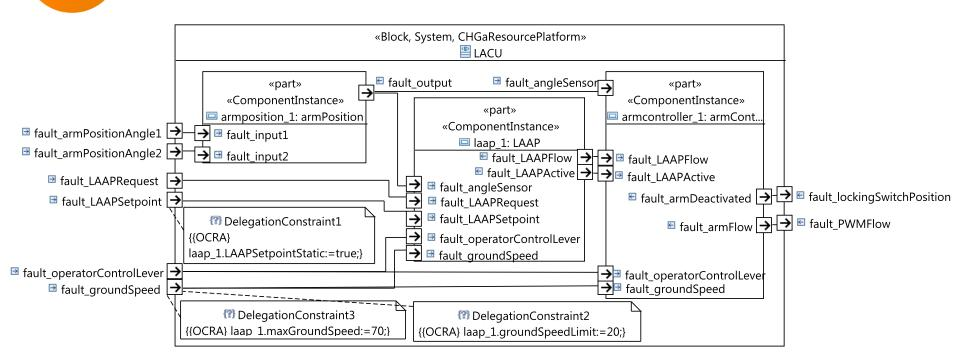
At this point we set the values of various configurable parameters used by the reusable component, e.g., LAAPSetpointStatic, maxGroundSpeed, groundSpeedLimit
